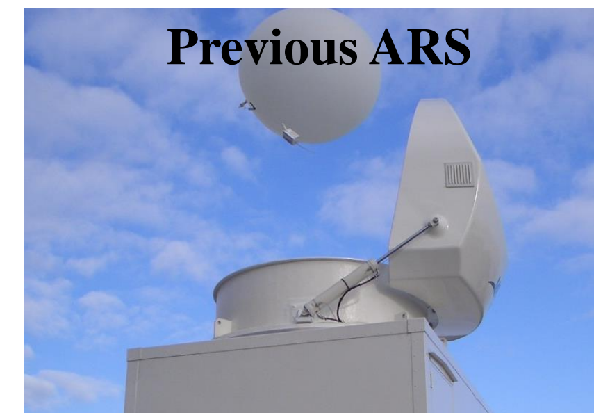
Turning wind shield hatch is effective but complicated mechanism
